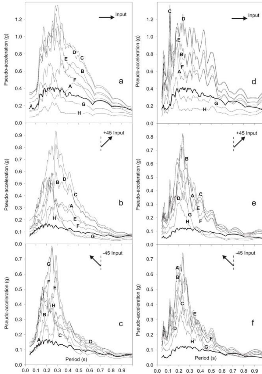
Fig. 10. Response spectra regarding “linear elastic analysis” imposing: (a) horizontal input; (b)  $+45^{\circ}$  inclined input; (c)  $-45^{\circ}$  inclined input. Response relative to “equivalent linear elastic analysis”: (d) horizontal input; (e)  $+45^{\circ}$  inclined input; (f)  $-45^{\circ}$  inclined input.
