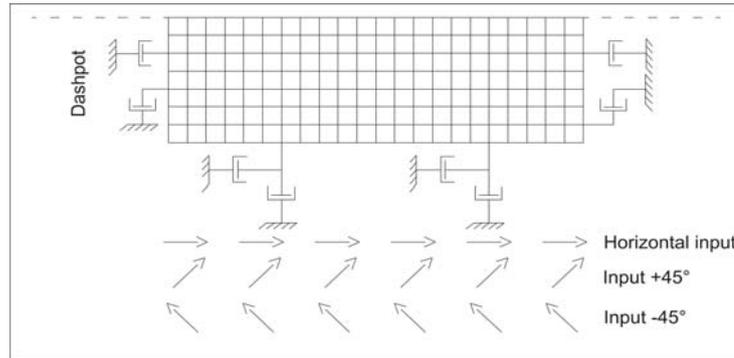
Fig. 2. FLAC numerical gridding with boundary viscous conditions and the selected directions of the seismic inputs.
