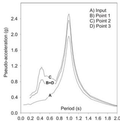
Fig. 6. FLAC spectra related to equation (5) with the evidence of identical responses of points 1 and 3.
