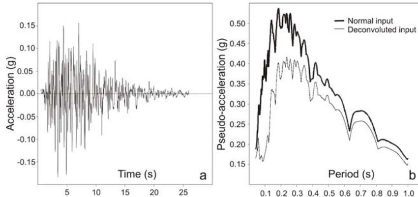
Fig. 3. Input accelerogram (a); normal and deconvoluted inputs spectra (b).
