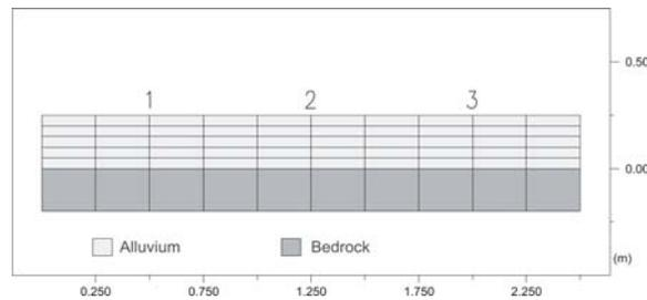
Fig. 4. Simplified testing section utilized to compare FLAC and QUAD4M results obtained at the three selected monitored points labeled 1, 2, 3.
