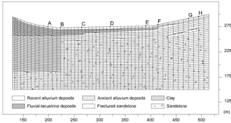
Fig. 1. Simplified modelling section with monitored points labeled A-H.
