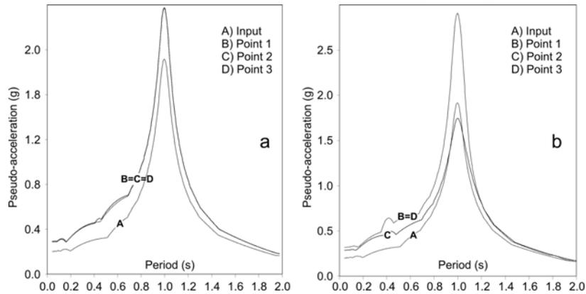
Fig. 7. QUAD4M spectra regarding equation (5): (a) seismic input only on the base, considering free the lateral boundary (the three points responses are identical); (b) seismic input both on the base and on the lateral boundary (responses of points 1 and 3 are identical).
