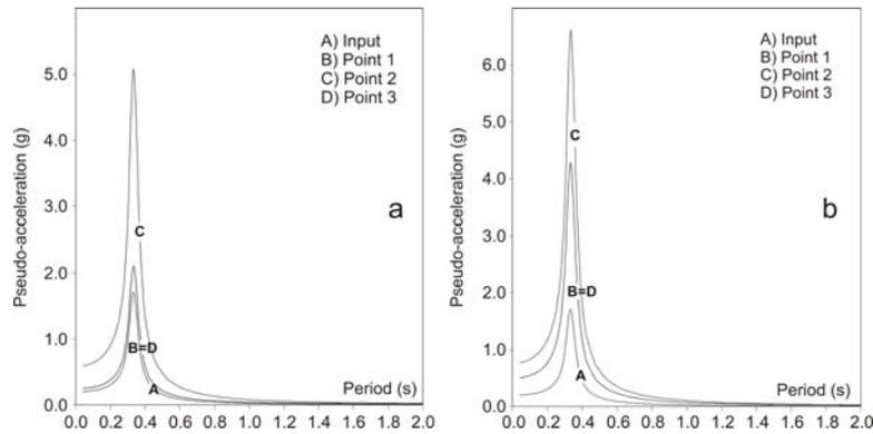
Fig. 9. QUAD4M spectra regarding equation (6), seismic inputs applied: (a) only on the base (responses of points 1 and 3 are identical); (b) both on the base and on the lateral boundary (responses of points 1 and 3 are identical).
